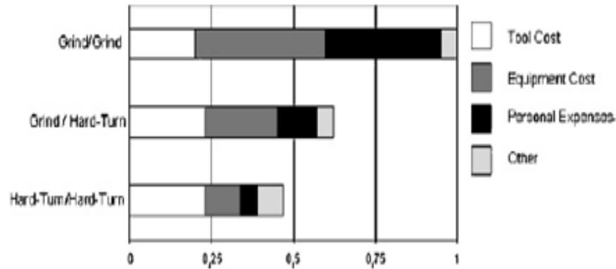
**Figure 1: Cost Comparison of Turning versus Grinding [3]**
